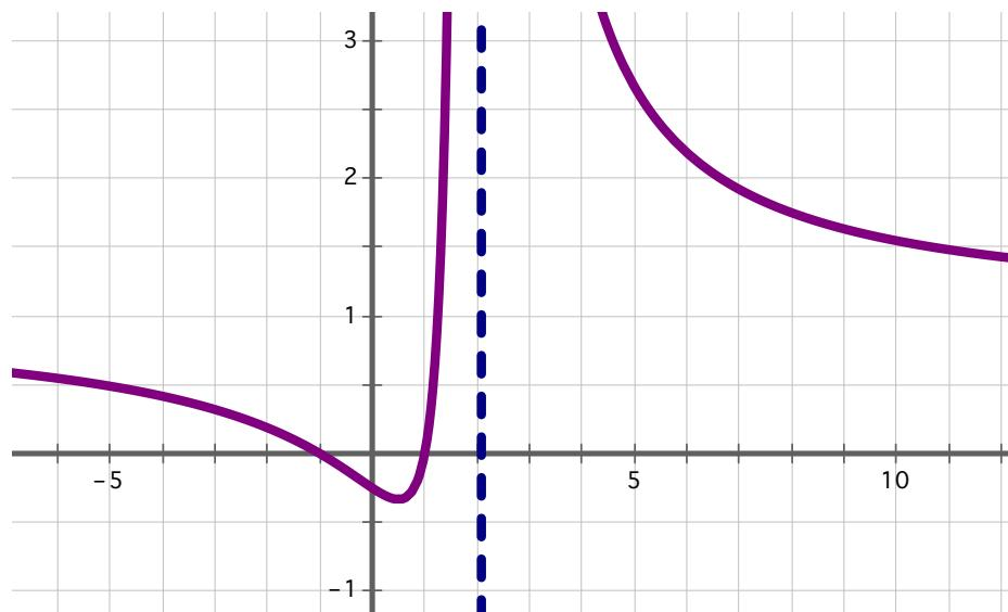
Notice what having two of the same factor in the denominator does to the curve: The curve goes up on both sides of the asymptote. Some calculators do not draw the vertical line in although it is there!!!
